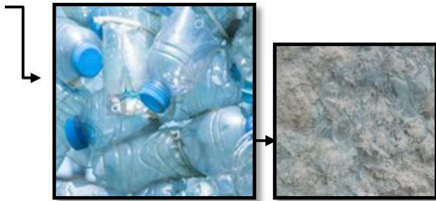
Figure 1. Pulverized high density PET materials.
